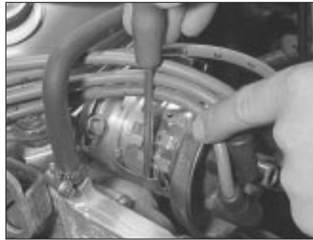
7.4b Releasing one of the distributor cap securing clips by carefully levering with a screwdriver
