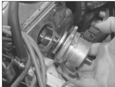
8.6 Removing the distributor from the cylinder head
