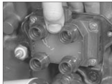
3.22 Distributorless ignition system ignition coil and mounting bracket removal (HCS engine shown)
