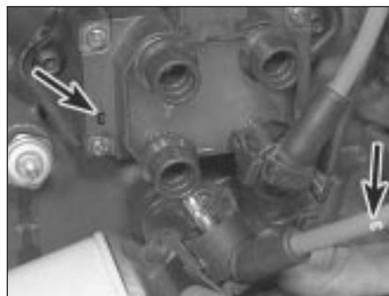
3.21 Removing an HT lead from the distributorless ignition system ignition coil. Note the corresponding markings on the ignition coil and HT lead (arrowed)
